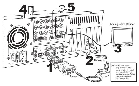
Figure 4. Extended Equipment Installation
